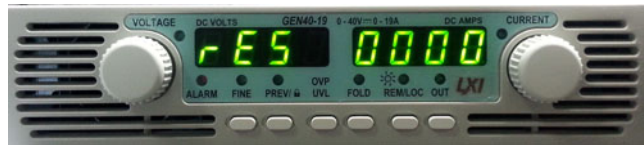
Fig. 6-8 External Power Supply - LAN Reset
