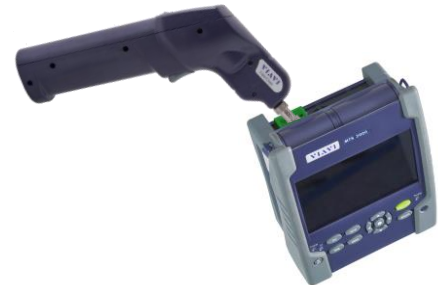
Figure 3: OTDR Port Inspection
