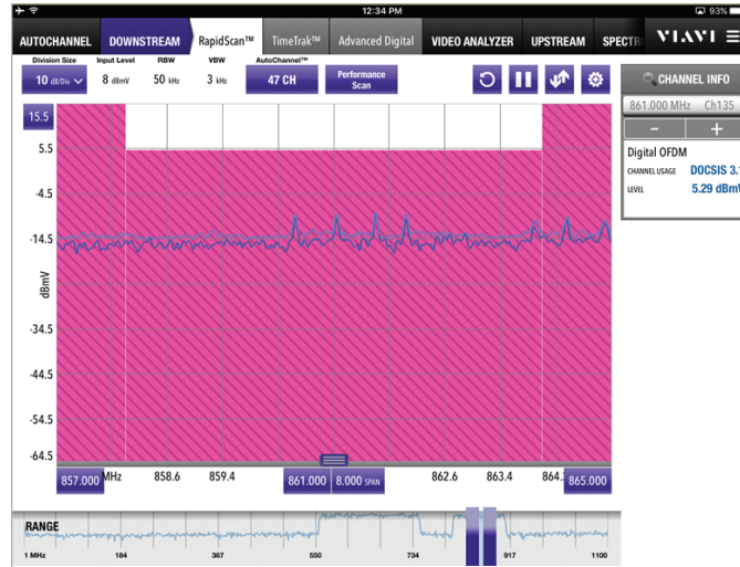
Zoom in to individual 6 MHz "block" within the OFDM signal with a "double tap."
